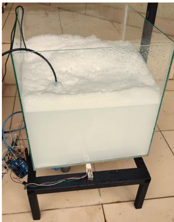
Figure 22: Apparatus for testing samples for DRC measurement
