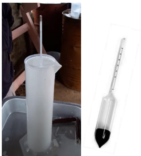
Figure 11 : Metrolac used for the DRC measurement
