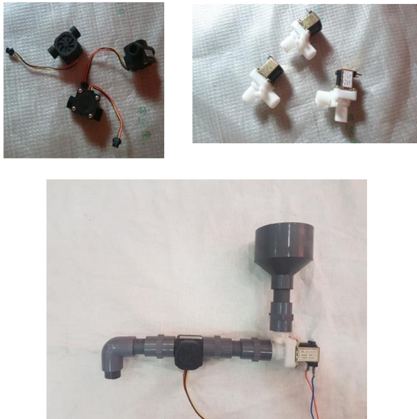
Figure 27: Flow meter and Electronic Solenoids
