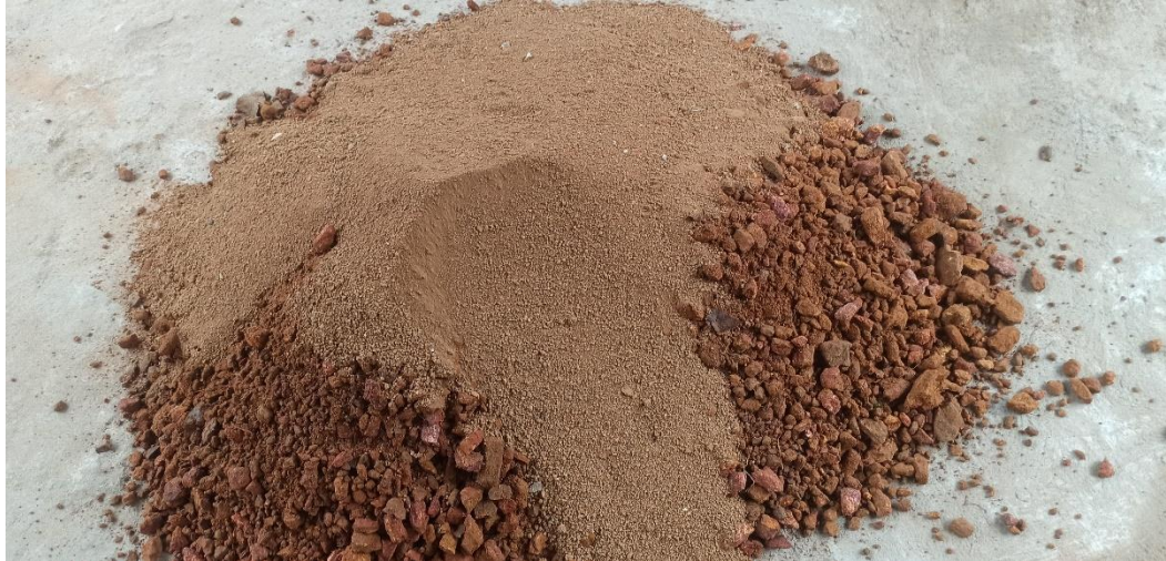
Figure 3-25: Soil proportions for the mixture
