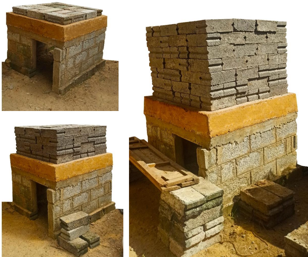
Figure 3-30: Loading procedure for the prototype
