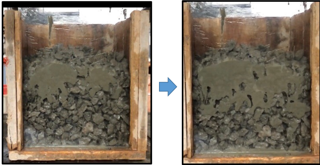
Fig. 3.1: Formation of smooth, thin cement paste layer on the surface
