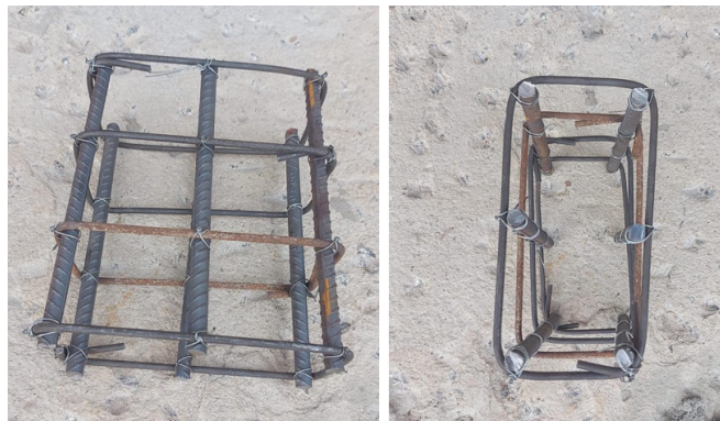
Fig. 5.2: Reinforcement arrangement of specimen with no honeycombs
