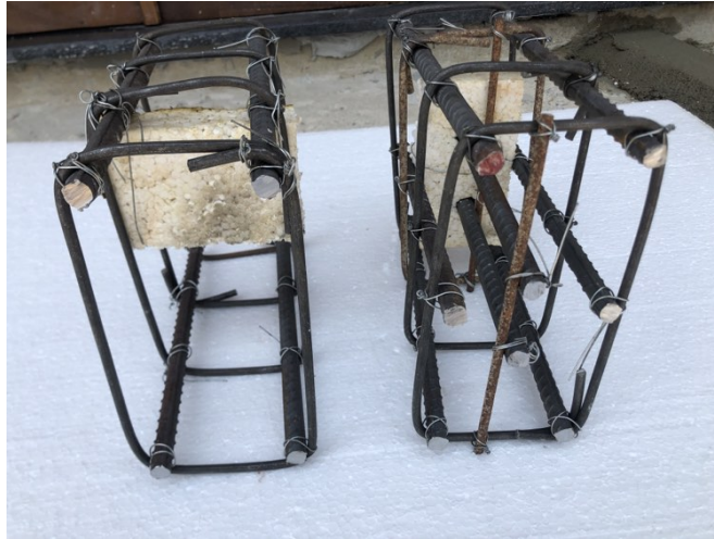
Fig. 5.5: Showing lightly (LHS) and heavily (RHS) reinforcement arrangement of specimen with honeycombs
