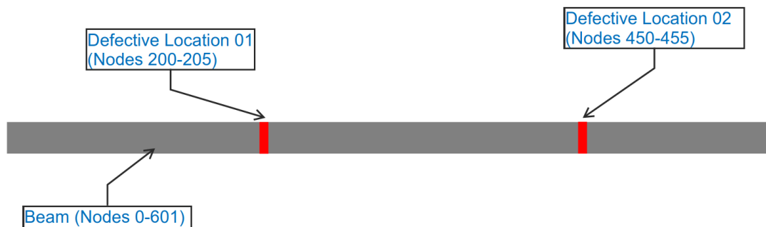
Fig. 7.10: Simulated defective locations in the beam
