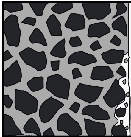
Fig. 3.6: Defects due to slurry leakage
