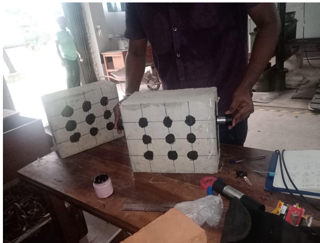
Fig. 5.6: Conducting the UPV test
