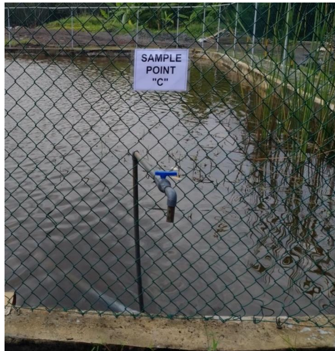
Figure 4-5: Location C - Near the outlet of the final treatment zone of the constructed wetland – water was collected through a bypass
