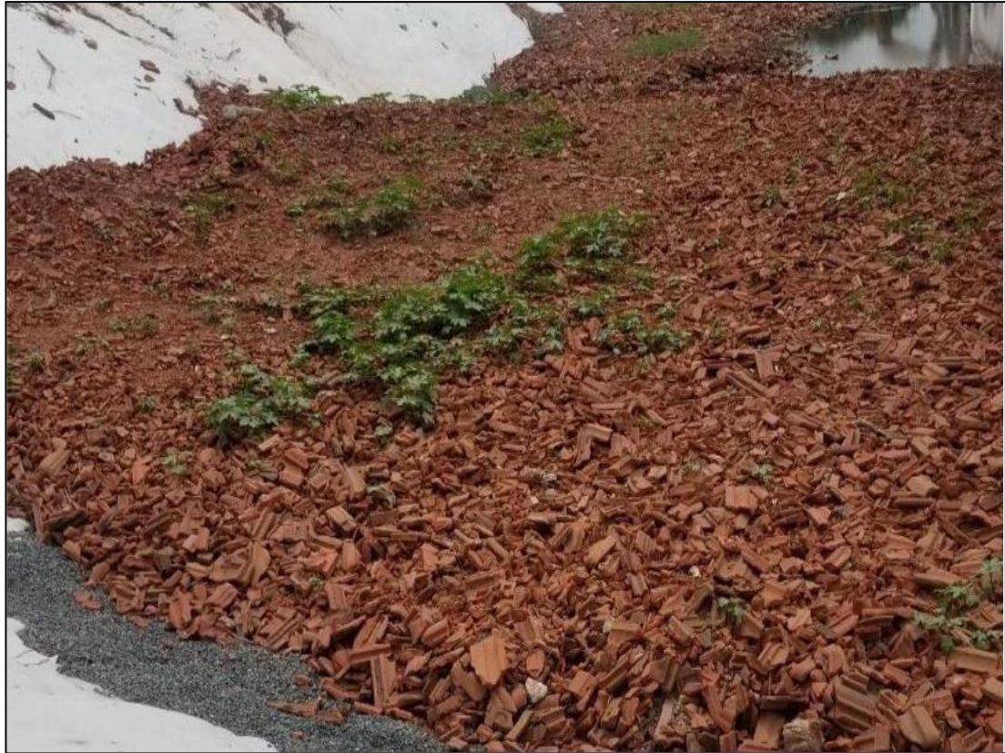
Figure 6-2: Broken burnt clay
