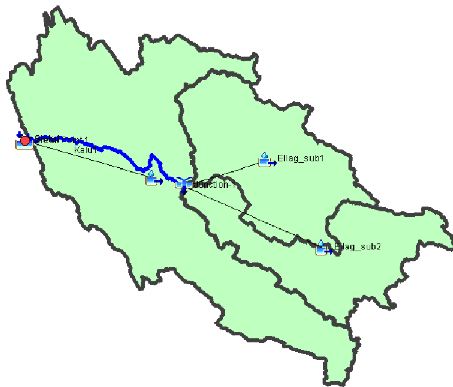
Figure 5-9: Kalu Ganga basin model with sub-basins developed in HEC-HMS
