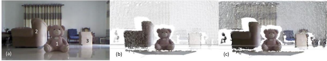
Figure 5.3: Effect of the distance to the point cloud density (a) RGB camera view of the scene. Selected objects are marked in numbers: (1) Bear – 2m from the camera, (2) – couch – 2.6 m from the camera, (3) – cardboard box – 4 m from the camera. (b) the point cloud displayed in 1mm points, (c) the point cloud displayed in 5mm points
