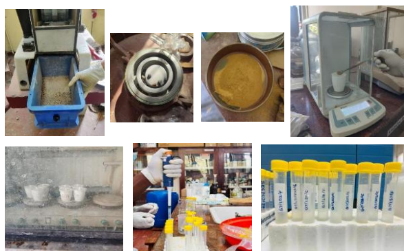
Figure 8: Sample preparation and digestion for ICP-MS
