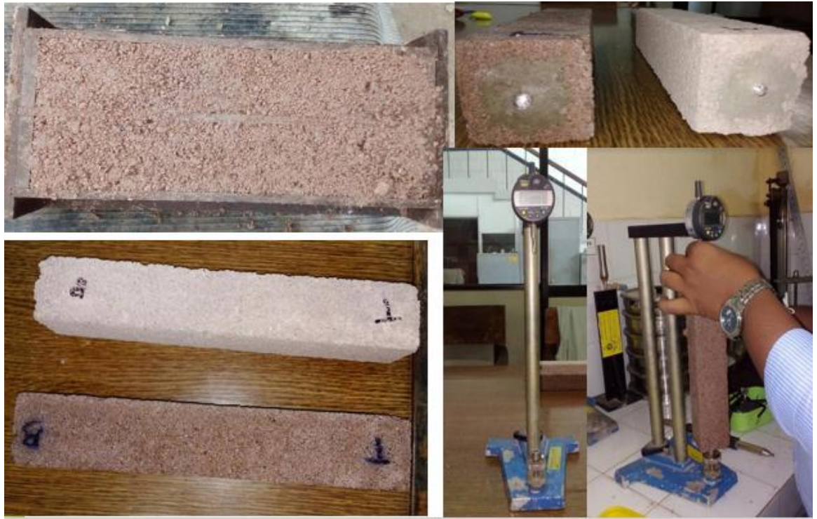
Figure 3-12: Wetting Expansion and Drying Shrinkage Measurements
