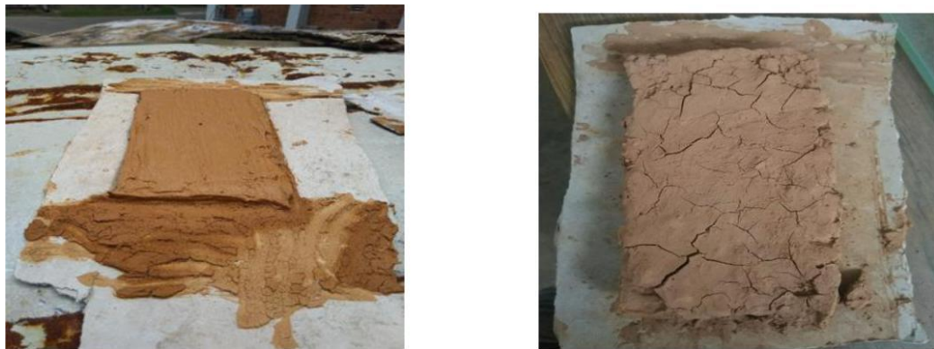
Figure 4-20: (a) Sample Casting and (b) after 24 hours of Casting
