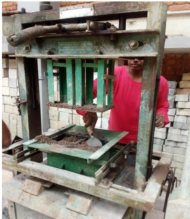
Figure 3-8: Use of Block Making Machine for CSEB Production
