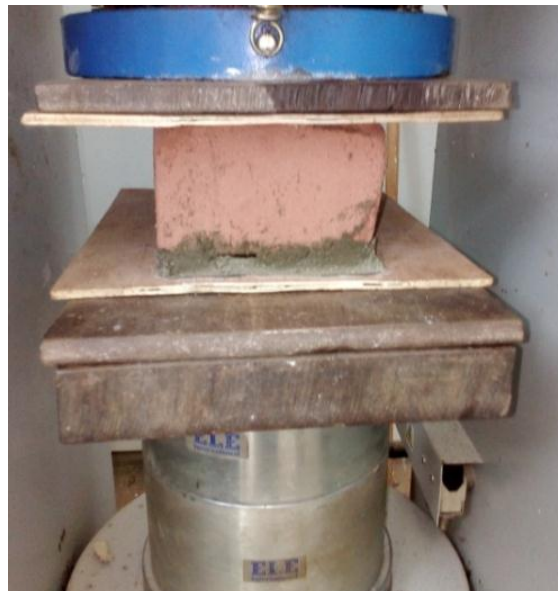
Figure 3-26: Testing of Bricks for Compression Strength
