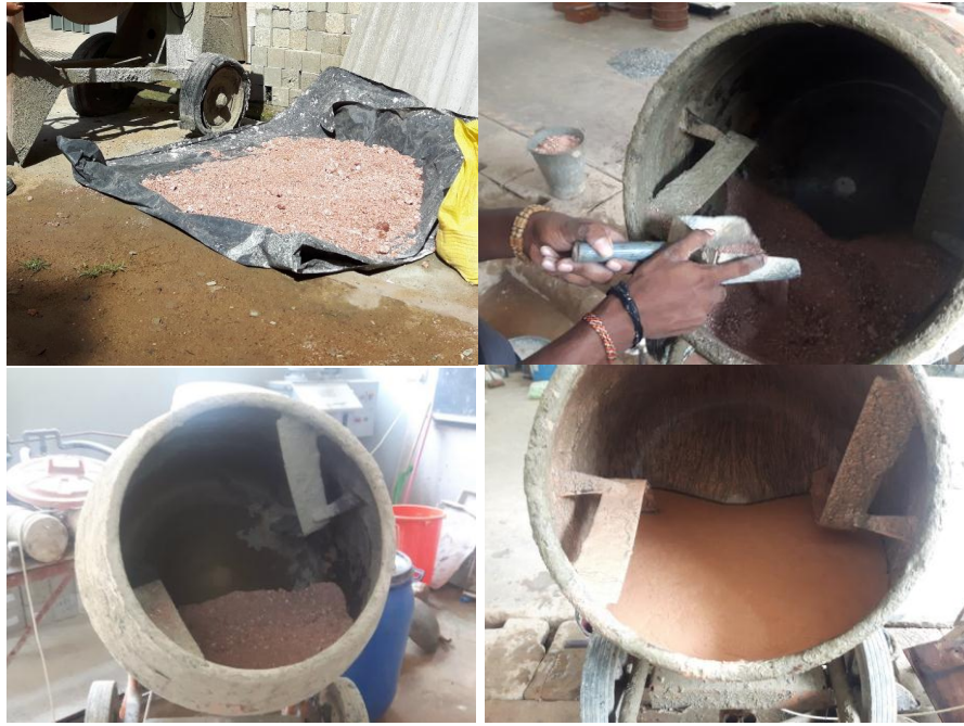
Figure 3-2: Use of Concrete Mixer for Soil Washing
