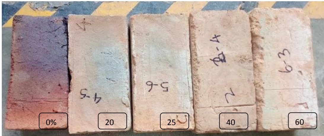
Figure 4-26: Burnt Bricks with Different Fly Ash Contents
