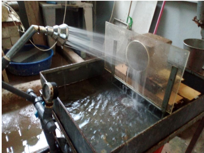
Figure 3-11: Accelerated Erosion Test Setup
