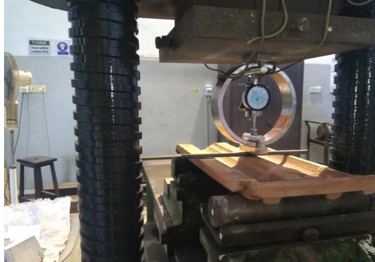
Figure 3-17: Transverse Strength Testing of Tiles
