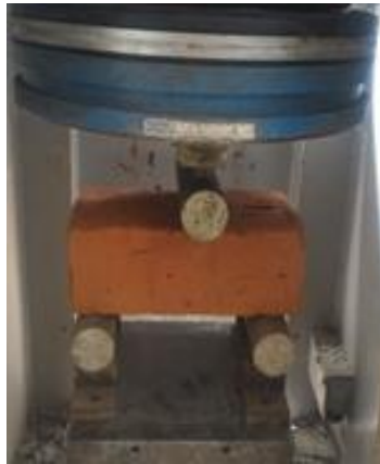
Figure 3-27: Testing of Bricks for Flexural Strength
