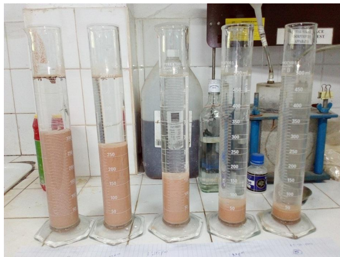
Figure 4-3: Amount of Sedimentation after 30 Minutes for Different Washing
