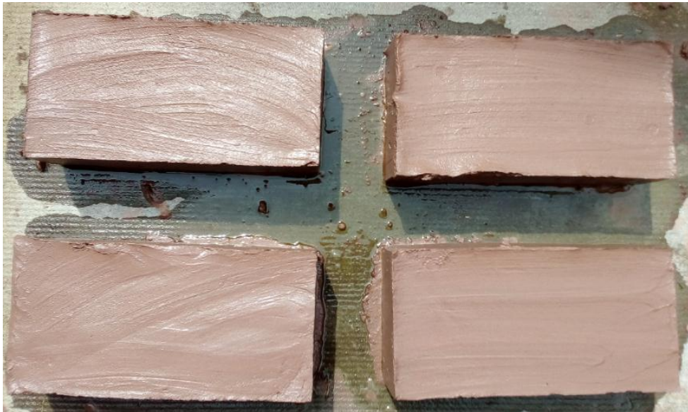
Figure 3-20: Prepared Bricks with Wooden Mould
