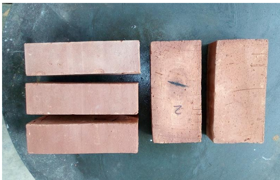
Figure 4-32: Wire-Cut Bricks made with Extracted Clay and Fly ash
