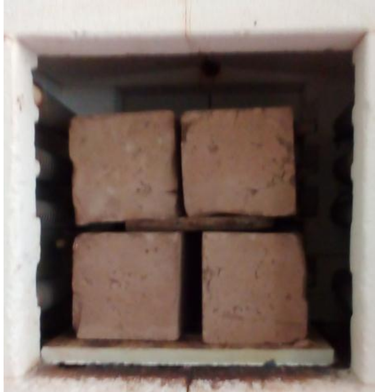
Figure 3-21: Burning of Bricks in the Furnace
