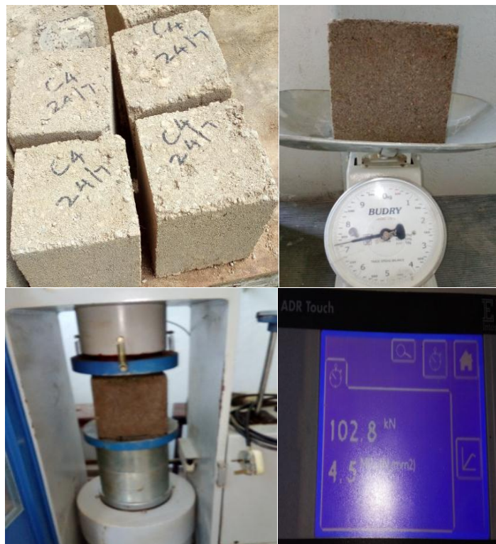
Figure 3-9: Cast Blocks and Compressive Test Procedure
