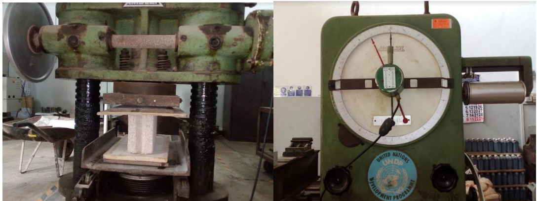
Figure 3-14: Use of Amsler Testing Machine for Compressive Strength Testing
