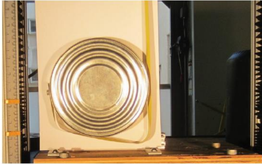
Figure 2.7: Experimental setup where the tape spring is enclosed around a cylinder (Wilson et al., 2020)
