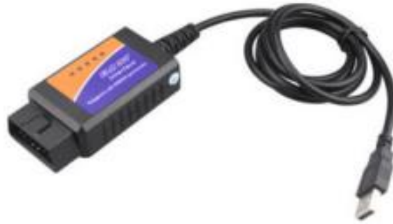
Figure 1: ELM327 OBDII to USB device used in the project
