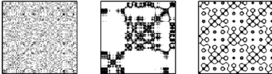
Figure 3.28 Sample Recurrence plots; totally random noise (left); random walk (middle); periodic composition of sine and cosine (right)
