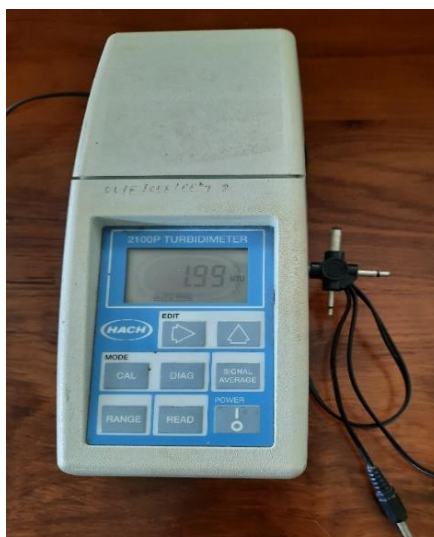
Figure 3.6: Turbidity meter (2100P)
