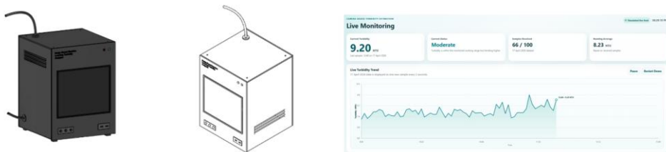
Figure 2: Conceptual hardware prototype (left) and software monitoring dashboard (right) for real-time turbidity estimation.
