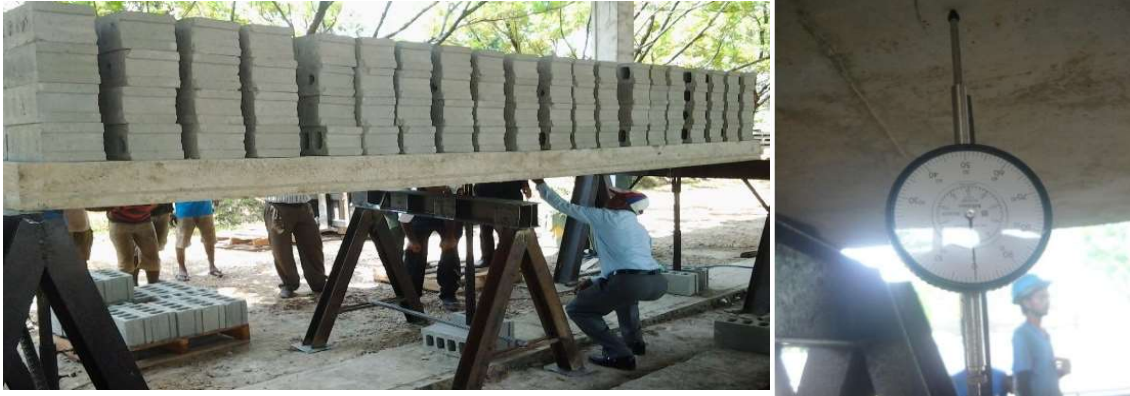
Figure 4.13: Load testing for sample slab
