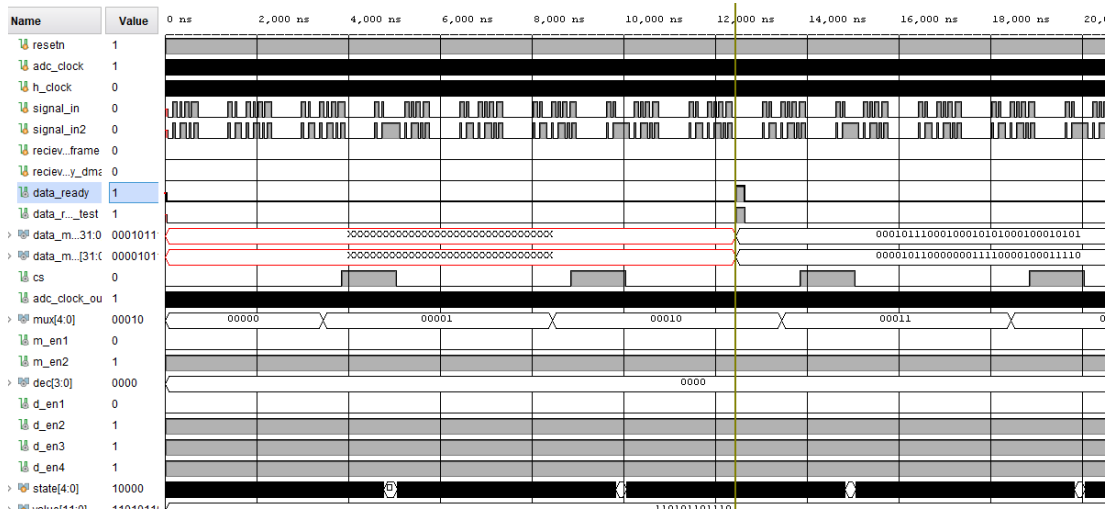
Figure 5.43: Simulation results for multiple ADC readings including all the input/output signals to and from the adc_0 module
