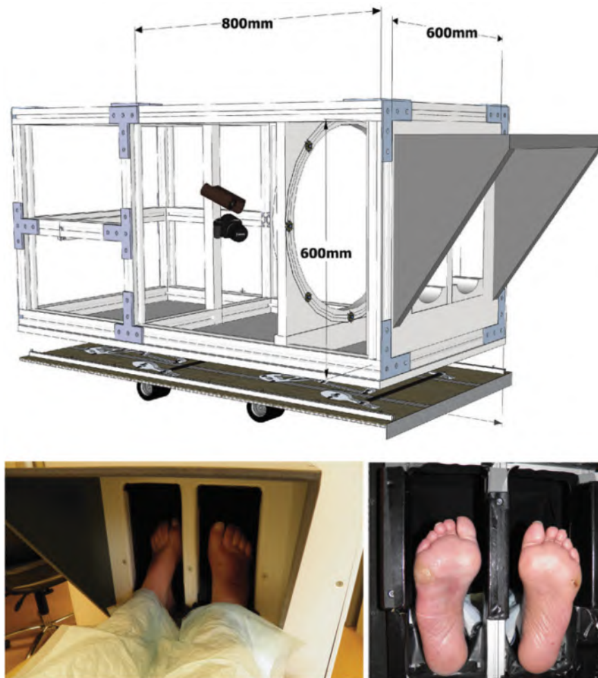
Figure 4.5: Experimental setup used by Van Netten et al. [151] for scanning foot plantar for diabetic foot complications
