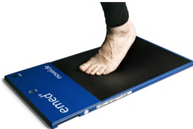
Figure 3.4: Electromechanical pedobarographic assessment tool for plantar pressure measurement developed by emed ® [83]
