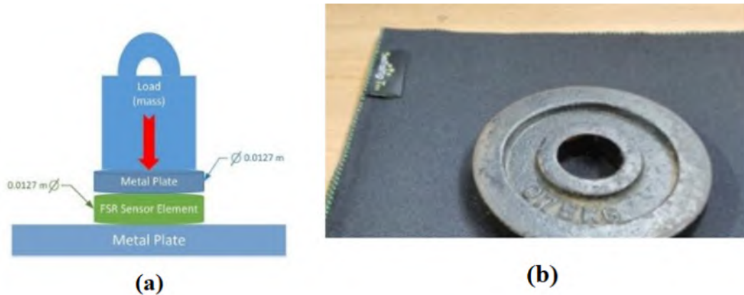
Figure 5.48: Static calibration techniques for pedobarographic systems with piezoresistive sensor arrays. (a) Calibrating individual sensels under different loading conditions using a Force Sensitive Resistor (FSR). (b) Placing individual weights discs of increasing mass
