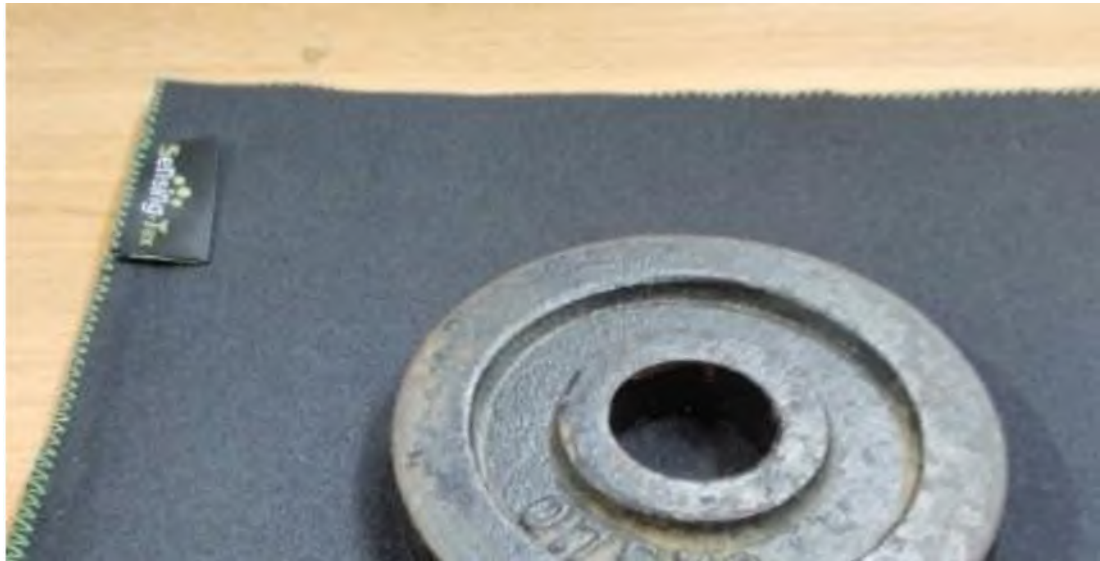
Figure 3.14: Metal disc which was placed on a SensingTex ® platform system to measure pressure distribution under two different loading conditions (static and dynamic) and using two different compensation algorithms
