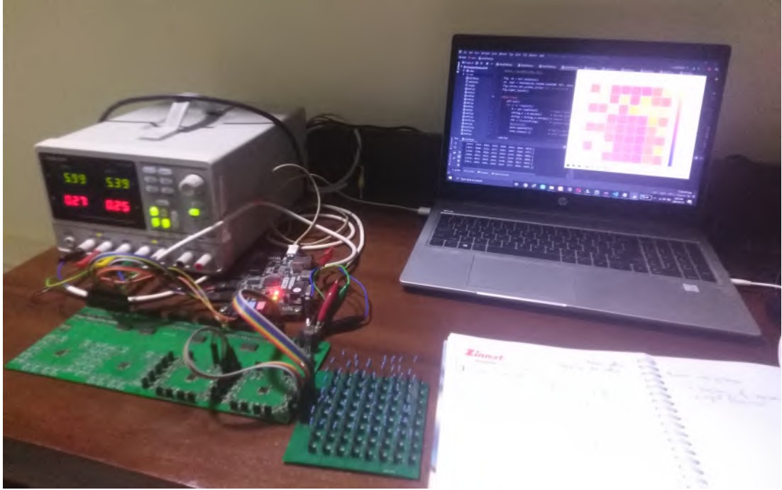
Figure 5.45: Development of the Python GUI program by debugging it with the 8 \times 8 RSA model
