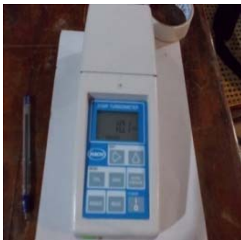
Figure 6.3: Digital Turbidity meter
