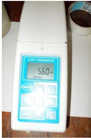
Figure 6.6: Reading given by the Turbidity meter
